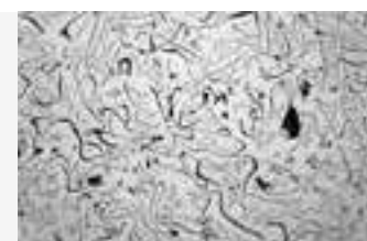
grey iron Excellent castability but brittle and not as strong
