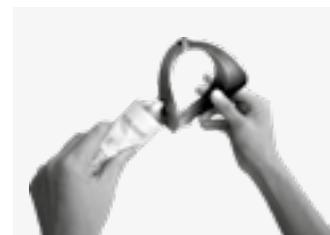
Check the colour code and make sure it is suitable for the intended use. Then apply a thin coat of VSH Shurjoint lubricant to the sealing lip of the gasket. The gasket supplied as standard is grade E (EPDM - green stripe), suitable for water applications.
