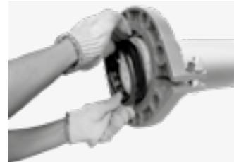
Fit the gasket in the gasket cavity between the outside of the pipe and the flange recess. Make sure that the bottom of the gasket (the marking side) is seated against the bottom of the flange recess.
