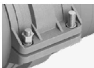
Thread a nut onto the end of each hex bolt until the washer makes contact with the coupling housing.
