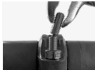
The installation bolt has a premachined slot. This allows the user to shorten the bolt, using pliers. The bolt can be easily shortened by bending the bolt back and forth several times. The shortened bolt makes insulation easy. This reduces the risk of the bolt sticking through the insulation material.
