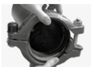
Pull the top and bottom halves of the coupling apart and remove them from the fixed pipe or fitting. (If the installation bolt is shortened, in most cases the coupling can be removed if the nut remains screwed 1 to 2 turns onto the
