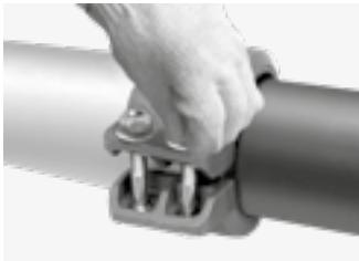
Insert the bolts and install a washer on each bolt end. Thread a nut onto each bolt and tighten the nuts by hand. Make sure that the oval neck of the bolt engages in the bolt hole of the housing.
