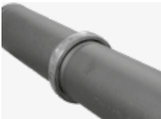
Bring the pipe together and align it with the opposite pipe. Push this pipe into the gasket until it touches the central lip. The gasket must not be in contact with the grooves in the pipes/fittings.
