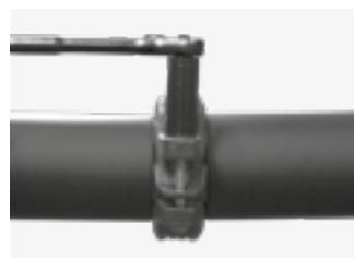
Tighten the nuts, starting with the installation bolt and alternating with the hinge bolt until the coupling parts and the wedge make metal-to-metal contact. See page 27 for correct torques.
