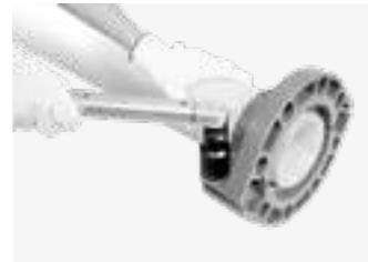
Tighten the drawbolts and nuts alternately and equally until the housing bolt pads meet and make metal-to-metal contact. Repeated alternate tightening will reduce the torque considerably.
