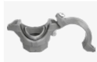
Fit the coupling housings loosely. Leave out one nut and bolt to allow for 'swing-over' installation.
