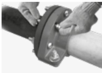
Add flange bolts and apply nuts hand tight. All the bolts shall be inserted from the same direction. Make sure that the oval neck of the bolt engages the bolt hole of the housing.
