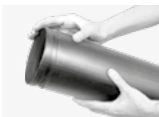
Ensure that the pipe is of the correct outside diameter and that rolled or cut grooves have been made correctly, according to instructions on pages 18-20. For optimum sealing, the outside of the gasket seating surface must be free of scratches, projections, rolling marks and other harmful defects such as loose paint, galvanising residue, soiling, chips, grease and corrosion.
