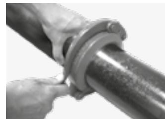
Firmly close the handle until it touches the back of the housing.
