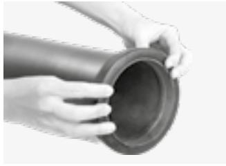
Fit the gasket on one end of the pipe so that the pipe end is visible. The gasket should never extend beyond the end of the pipe.
