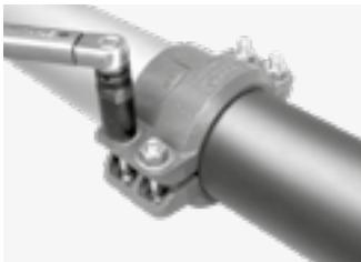
Tighten the nuts alternately and equally until the bolt pads meet and make metal-to-metal contact. Repeated alternate tightening will reduce the torque considerably. Tighten the nuts by another quarter to
