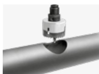
Determine the location for the hole on the pipe. Use the correct holesaw size as stated in table on the next page.
