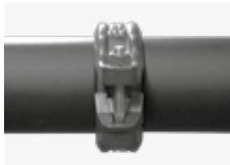
Only **loosen** the installation bolt until there are 2-3 threads visible above the nut. The bolt and nut do not have to be removed completely, as they hold the coupling parts and the wedge together.
