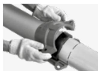
Place the housings over the gasket, ensuring that they remain centred between the first set of marks. Ensure that the housings remain centred between the second set of marks and that the tongue and groove fit together correctly.
