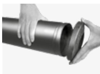
Fit the larger opening of the gasket over the larger pipe end and align the two pipes to be coupled. Insert the smaller pipe into the gasket. A slight twisting motion of the pipe will make assembly easier. The gasket must not extend beyond the end of the pipe or beyond the grooves of both pipes.
