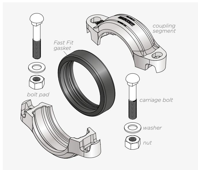
The VSH Shurjoint Model SS-1200 is designed for high pressure applications including reverse osmosis and desalination systems. The coupling is supplied as standard with a special VSH Shurjoint Fast-Fit gasket, type 316 carriage bolts, washers and silicon bronze nuts. The SS-1200 working pressures are exclusively based on use with cut groove pipe ends.
