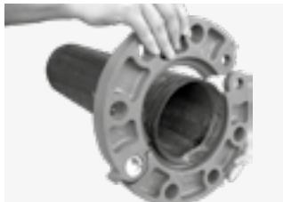
Fully open the hinged flange segments. Fit the flange segments around the groove of the pipe end and pull the segments together until the holes are aligned.
