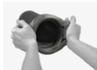
Install the coupling on the grooved pipe end or fitting. Make sure that the centreline of the gasket is aligned with the centreline of the fitting and press the coupling evenly until the gasket is positioned over the grooved end. Then install the other pipe end in the coupling. The gasket has a central lip which stops the coupling when correctly positioned. Visually check that the keys of the coupling are aligned with the grooves.
