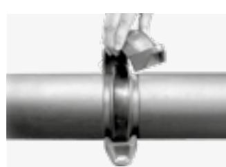
For 'swing-over' installation, place one of the coupling housings over the bottom of the gasket and swing the other coupling housing into position over the top of the gasket. For standard installation, fit the coupling housings over the gasket one at a time. In both cases make sure the coupling edges are fully engaged in the grooves.
