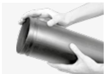
Ensure that the pipe is of the correct outer diameter and that rolled or cut grooves have been made correctly, according to instructions on pages 18-20. For optimum sealing, the outside of the gasket seating surface must be free of scratches, projections, rolling marks and other harmful defects such as loose paint, galvanising residue, soiling, chips, grease and corrosion.
