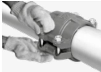
Fit a washer on the end of each bolt. Thread a nut onto each bolt and tighten the nuts by hand. Make sure that the oval neck of the bolt is entirely countersunk in the bolt hole of the housing.
