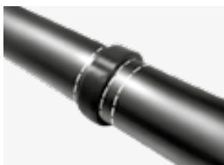
Place a gasket over the pipe ends and centre the gasket between the first set of inner markings. The pipe ends must always be in contact with each other.
