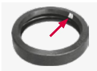
Check the colour code of the gasket and that it is the correct one for the intended use. The gasket supplied as standard is grade E (EPDM, green stripe code), suitable for water applications.
