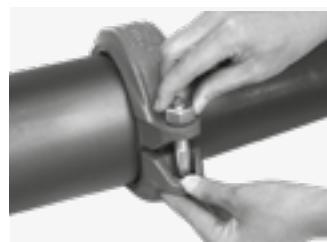
For 'swing-over' installation, insert the remaining bolt and turn the nut hand tight. For standard installation, insert both bolts and turn the nuts hand tight. Make sure that the oval neck of the bolt is entirely countersunk in the bolt hole of the housing.
