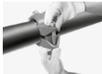
Fit the bolts and turn the nuts hand tight. Make sure that the oval neck of the bolt is entirely countersunk in the bolt hole of the housing.
