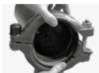
Pull the top and bottom halves of the coupling apart to release the coupling key from the groove. Then remove the pipe or fitting from one side of the coupling.
