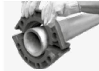
Fit the flange housings with the machined teeth onto the HDPE pipe end. The gasket cavity must point towards the pipe end. Insert the drawbolts into the flange adapter housings. Install a washer onto the end of each bolt. Thread a nut loosely onto the end of each drawbolt.
