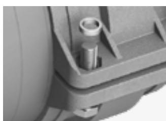
Fit a hex bolt and a washer on each end of a bolt hole in the housings. Make sure the head of each hex bolt and washer is properly seated in housing recess.
